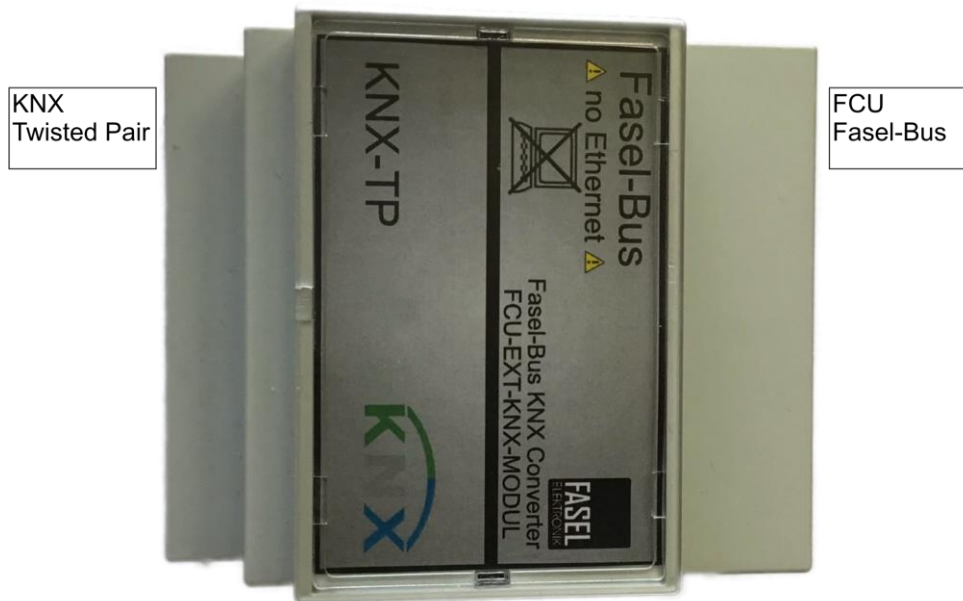
Connections of the KNX Module.
