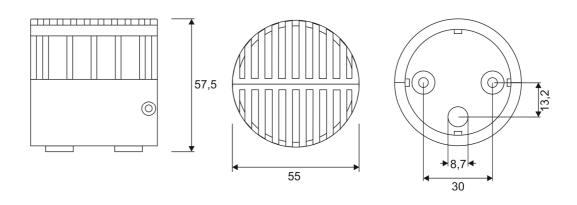
Stove sensor temperature with safety temperature control fuse (STB 141°C +0/-5°C) (FCU-SENSOR-OVEN-A)
